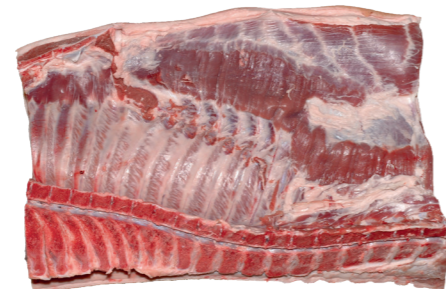
The middles have to be aligned and with the loin at the robot side before transfer to the inlet
